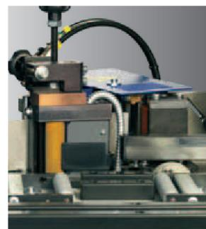
The knurled glue roller ensures an even application of glue to the workpiece. The 1.2 kg glue pot provides sufficient glue capacity.
