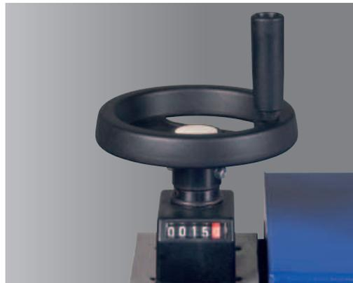
Workpieces from 10 to 45 mm in height can be machined.
